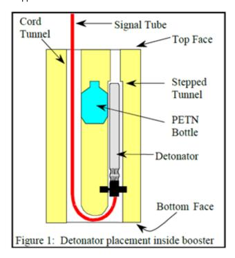
The cord or tube downline should be kept taut during charging and stemming, to prevent damage and minimize abrasion. However, if a primer begins to float on top of a rising column of bulk explosive, temporarily slacken the downline. Once the surface of the explosive column has risen past the primer, tension can be reapplied to the downline.
